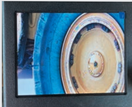
Tyre handler still in the same position with half zoom activated on the truck 8 Metres away.
