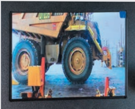
Standard vision looking at the truck parked 8 Metres in front of the tyre handler.
