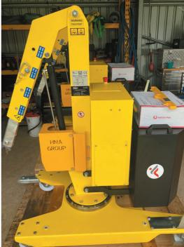
HNA Group have designed, developed, manufactured, and patented the Model 01B2 Swivel Crane which allows lifting and handling of loads of up to 200 kg. Crane rotates 360° with free rotation (lever in rest position) or can be locked every 30° (lever actuated) by means of a slewing ring at the base of the column.
